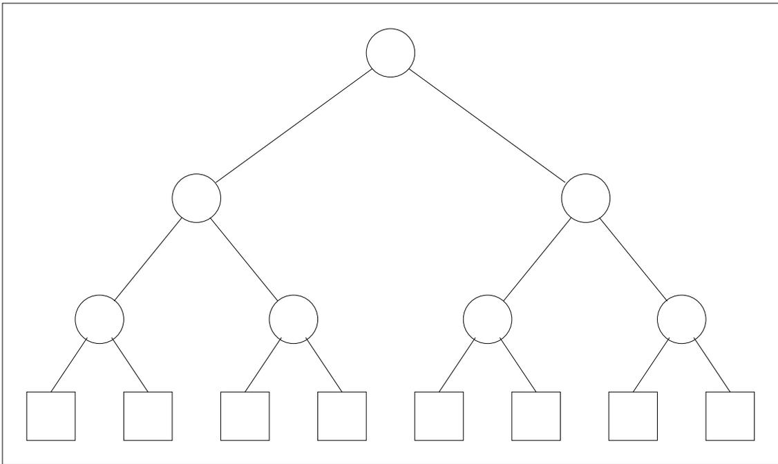
Figure 5.6 An FFP Machine with Eight L-cells
